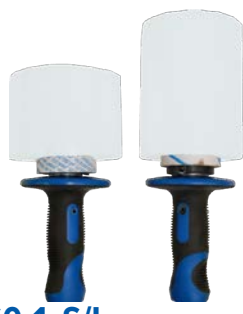
EP-760-1 S/L Hand Film Dispenser - Short/Long Film Roll Options: 3" (short) or 5" (long) Core ID: 1 1/2" Tension adjustable Ergonomic pistol handle
