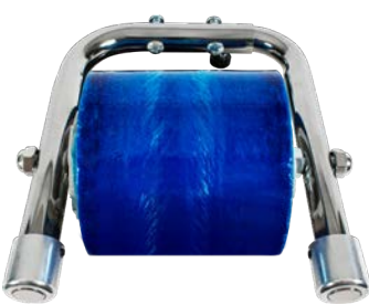
EP-765 Hand Bundling Dispenser Film Roll Range: 3" & 5" Core ID: 3" Tension adjustable Magnetic attachment
